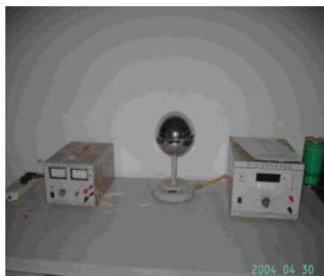
图 1-1 YQF-1 型圆球导热系数测定仪 Fig.1-1 YQF-1 type thermal conductivity spheroid instrument
